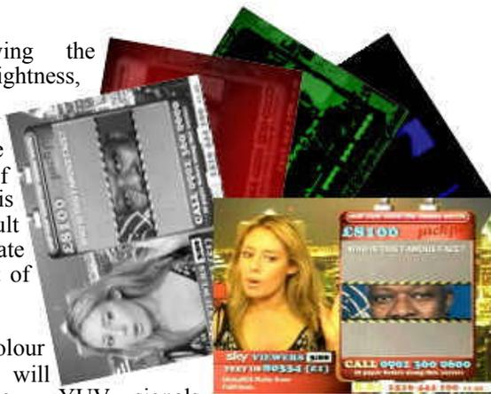
So your colour television will receive the YUV signals (brightness, red difference, blue difference) and from this create the RGB (red, green, blue) signals necessary to drive the three cathode emitters in the television tube.
